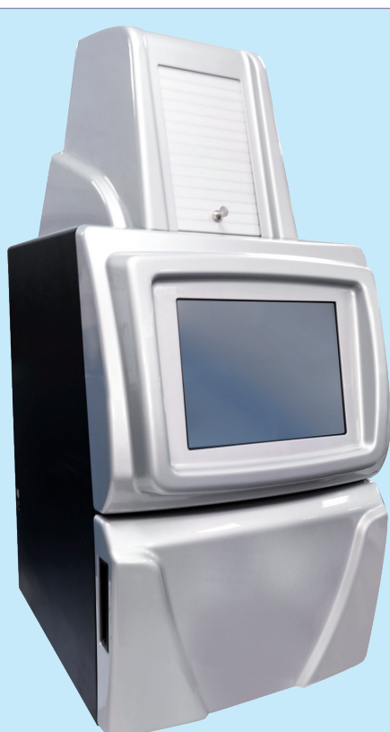
FastGene® FAS-V: High-end gel documentation system with very light-sensitive 2 MPixel CCD camera, XXL-transilluminator, built-in computer & 10,4" touch screen control.
