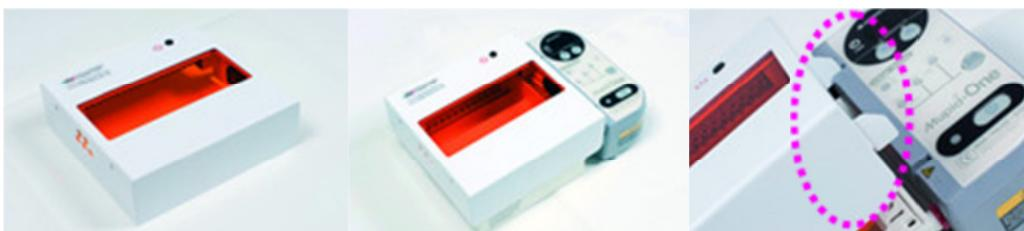
**Step 4: Make sure the power safety buttons of *Mupid™ One* have been pressed by the 2 hooks on sidewall of the MUPID™ LED Illuminator**
