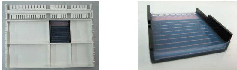
**Step 2: Put the gel with gel tray in Mupid™ tank and perform dye loading**
