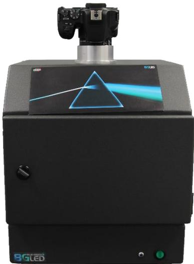
Place a gel on the transilluminator and switch on the device. Attached the cover plate on the observation window to avoid scattered light. Set up the camera with the recommended camera settings (p. 10). Take a picture by pressing the shutter release. Change the camera settings if the picture is not satisfying. Pictures are saved on the SD card.
