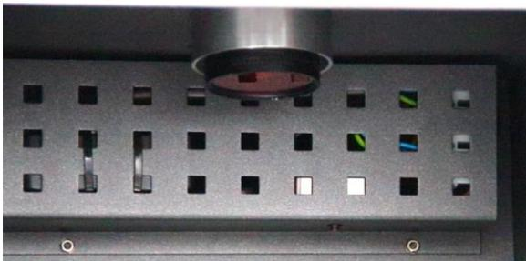
Extend the lens barrel by zooming out. The lens is now exposed and the filter is ready to be removed. The filter is held in place using a magnetic filter holder. After removing the filter, add the white light source (e.g. FG-07CE).
