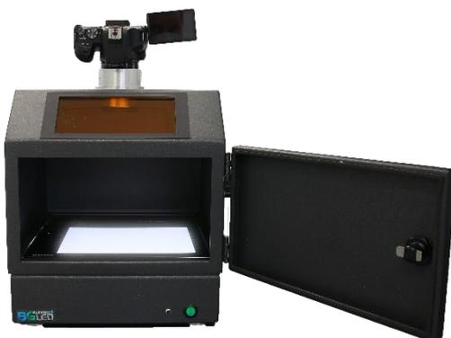
Add the white LED transilluminator to the central area of the Blue/Green LED Transilluminator DE as shown in the picture and place the cover plate on the observation window. Turn the switch to battery. Make sure that the transilluminator is charged, otherwise connect the transilluminator to a power source using the USB charger cable. Select the required brightness by pressing the switch button. Record your image.
