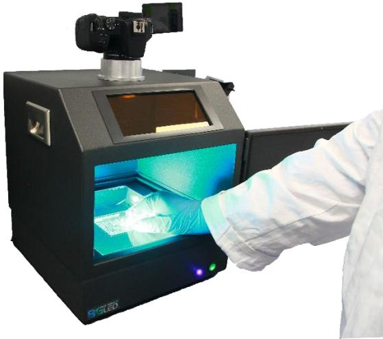
Turn on the transilluminator and remove the cover plate. Now look through the observation window and excise the DNA band using a scalpel or our FastGene® Agarose Gel Band Cutter (FG-830). Please keep in mind, the usage of a scalpel can damage the glass plate of the transilluminator, which can lead to artefacts in the pictures.
