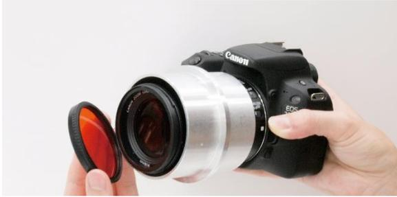
Recording images of protein gels or petri dishes are possible by adding a white light source and removing the FastGene® amber filter from the lens. The procedure is shown in the next steps
